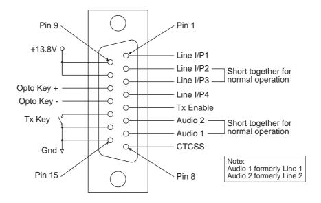
Figure 1.5 T856/857 D-Range Wiring - Rear View
