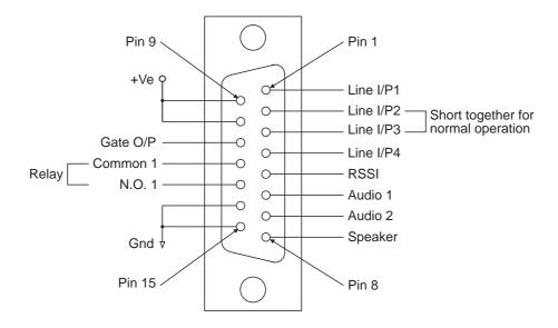
Figure 1.4 T855 D-Range Wiring - Rear View
